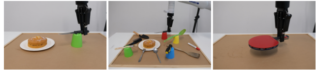
Fig. 9: Illustration of accuracy, robustness, and generalization evaluations. The accuracy evaluation requires the model to recognize the affordance of a single object and execute related task. The robustness evaluation involves accurately selecting an object in a cluttered scene to perform a specified affordance task. The generalization evaluation assesses if the model can reason about the graspable area of unseen objects.
